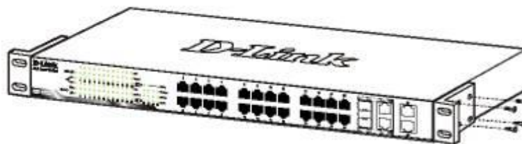
Figure 2.2 – Attach the mounting brackets to the Switch
